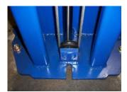
Be sure cables are seated securely on the sheaves.
