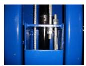
Cables are routed identically the same on both columns. Cable on right is routed down and around the sheave then up and over the overhead beam. Then routed down to the top of the carriage.
