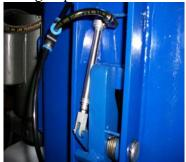
4. Attach palm valve to steel bracket on side of column.
