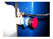
5. Connect shop air to palm valve. We recommend using leftover hose and NPT fitting (not included).
