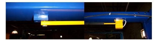
**4.** Run electrical cord into the beam and back out of the column using provided bulk head fittings.
